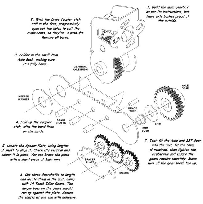
8. Slot the completed unit over the gearbox axle bush. Add the Keeper Washer over the bush, push it towards the gearbox, so there is minimal clearance. Solder the washer to the bush only, leaving the coupler unit free to swing.
