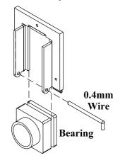
The completed assembly can now be soldered to the inside face of the chassis, using axle jigs. If you fit it with the bearing in place,make sure the sliding surfaces are lightly oiled, to prevent the bearing being soldered to the etch.
