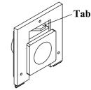
The tab is designed to sit exactly 4mm above the axle centre line, with the loco on level track. The top edge of the cut-outs on most chassis is also 4mm above the axle centre, so the tab can be butted against the top of the cut-out to set the unit at the correct height.
