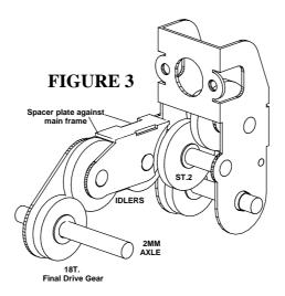
Noting their locations and number of teeth, (they are not interchangeable) fit the two **Idler Gears** (loose-fit on 2mm shaft) into the **Swinging Arm Assembly**, along with their short gearshafts, and secure as above. The larger bosses on the gears should run against the Spacer Plate, as shown in Figures 2 and 3.
