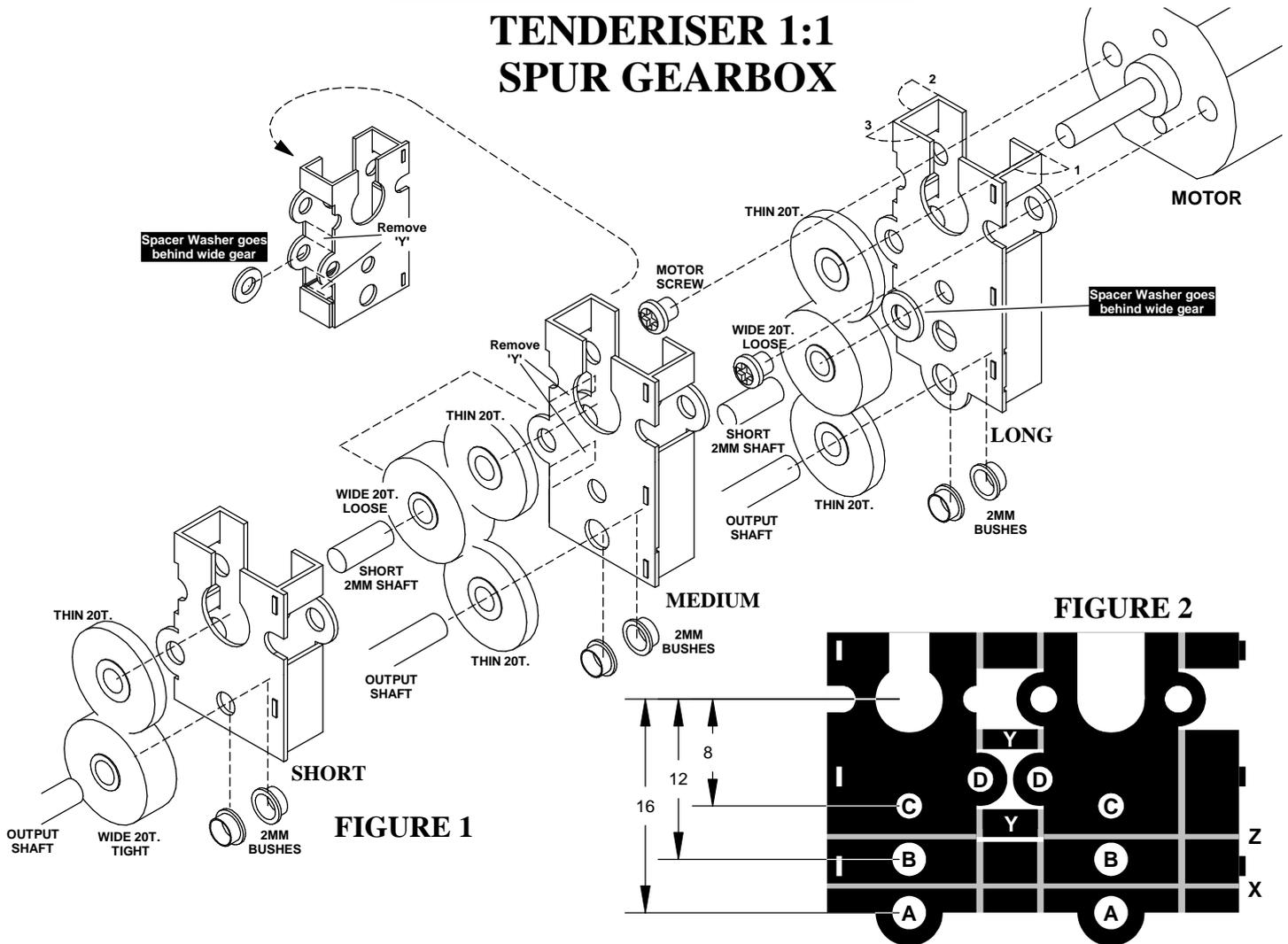
Remove the gearbox etch from the fret, then study Figures 1 and 2 and decide which configuration you're going to build.
