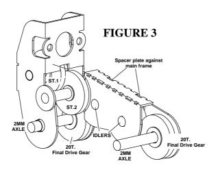
Now fit the 20 tooth **Idler Gears** (these are a loose-fit on their shafts) into the **Swinging Arm Assembly**, along with their short gearshafts, and secure as above. The larger bosses on the gears should run against the Spacer Plate, as shown in Figure 2.
