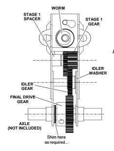
12. Fit the motor/worm assembly, (L) check the mesh (M) and test the gearbox under power. Lightly lubricate the mechanism (N) then the gearbox is ready to fit (C & J).
