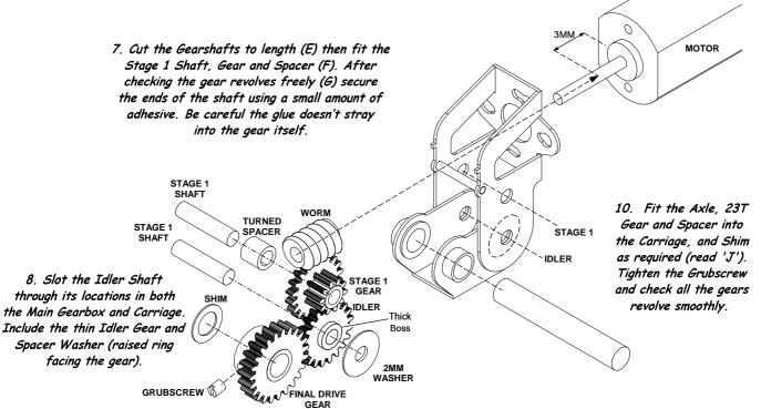
9. The Final Drive Carriage can be sited anywhere on its arc, facing either way, but it must be fixed in place before applying power (Section 'H').
