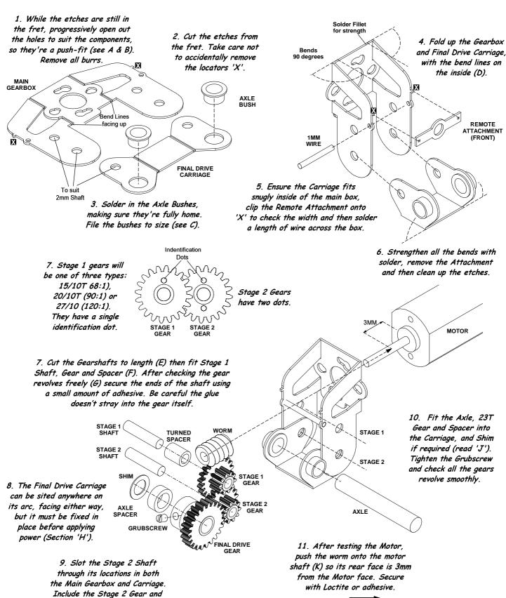
check the double gears run freely, with some side clearance (G).
