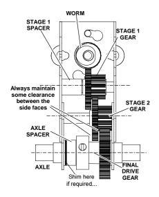
12. Fit the motor/worm assembly, (L) check the mesh (M) and test the gearbox under power. Lightly lubricate the mechanism (N) then the gearbox is ready to fit (C & J).
