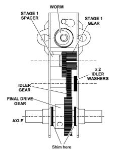
11. Fit the motor/worm assembly, (L) check the mesh (M) and test the gearbox under power. Lightly lubricate the mechanism (N) then the gearbox is ready to fit (C & J).
